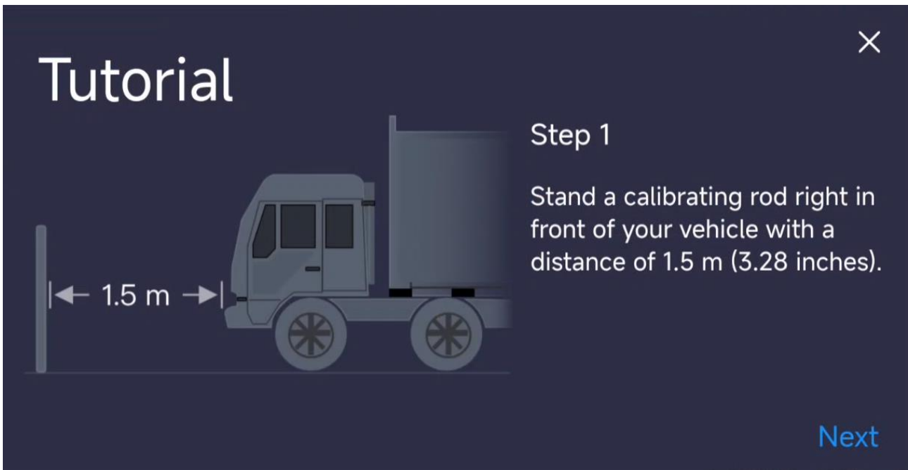
Figure 15-9 Calibration Step 1: Calibration Rod
