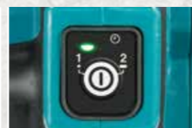
Main power switch with auto power-off function
